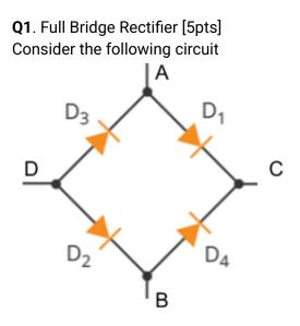
Here is a plot of the voltage difference  $V_a$ - $V_b$  as a function of time (e.g. due to having A and B connected to an AC voltage source). On top of this plot, draw the line corresponding to  $V_c$ - $V_d$  (e.g. imagine you are measuring it with a voltmeter while nothing else is connected there). Assume the forward voltage drop of the diodes is zero.
